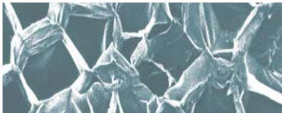
Photo: Cell structure of EPS under a microscope
